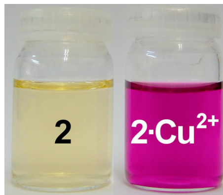
Figure 6. Visual changes in the colour of 2 (left) after addition of \text{Cu}^{2+} metal cation (right).
